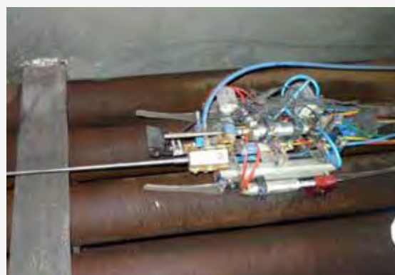
Figure 4. ROV on the top of the bundle.
